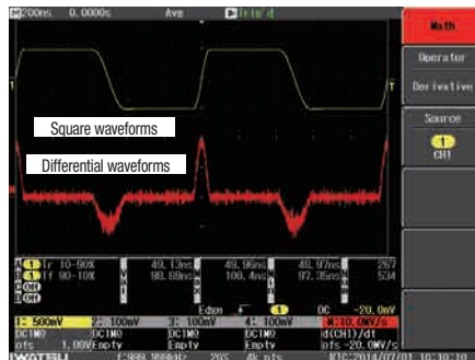
Differential calculation waveforms for square waveforms (rising 50ns, falling 100ns) (Displays the size of the time fluctuations (dv/dt) for square waveform edges.)
