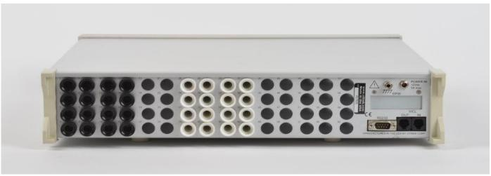
The 964i rear panel accommodates up to 60 output terminals. Unit shown above with 16 + terminals (HV) and 16 – terminals (return). The 964i ships with mating connectors for all +/- HV terminals 7KV and higher. Custom length HV lead sets are optionally available.
