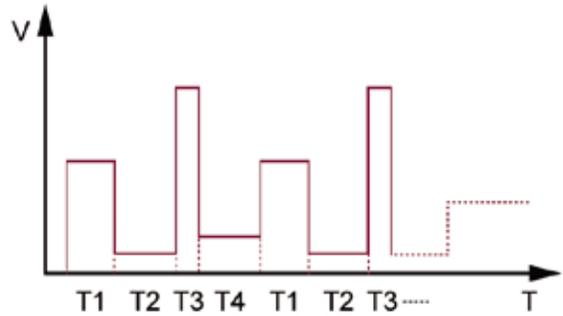
List mode allows user to create a sequence of steps, store it into the power supply's non-volatile memory and execute it. The input parameters for generating a list include the name of the list file, the input steps (no more than 150 steps), the step time (the minimum is 100mS) and the value of each step.
