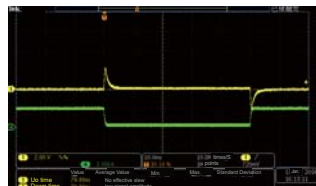
8 sets of IT6522C paralleling together Voltage ratings: 10V, Current ratings: 960A Load current: Level B=100A Level A=800A F=10Hz
