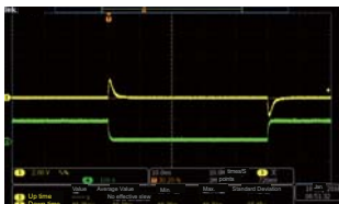
Standalone set IT6522C, 80V, 120A, 3000W Voltage ratings: 10V, Current ratings: 120A Load current: Level A=10A Level B=100A F=10 Hz
