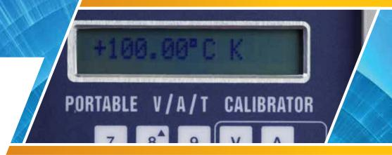
Thermocouple simulation allows the fine tuning of any measurement or control loop. Temperature measurement is automatically compensated for the cold junction temperature.
