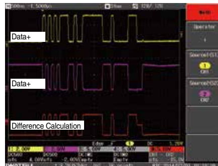
Measuring Differential Serial Signals
