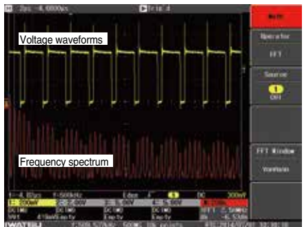
Frequency spectrum analysis (FFT calculations of switching voltage waveforms).
